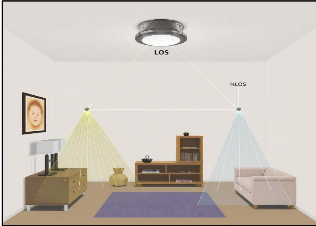
Fig 2: LOS and NLOS Propagation Paths in Li-Fi Systems
