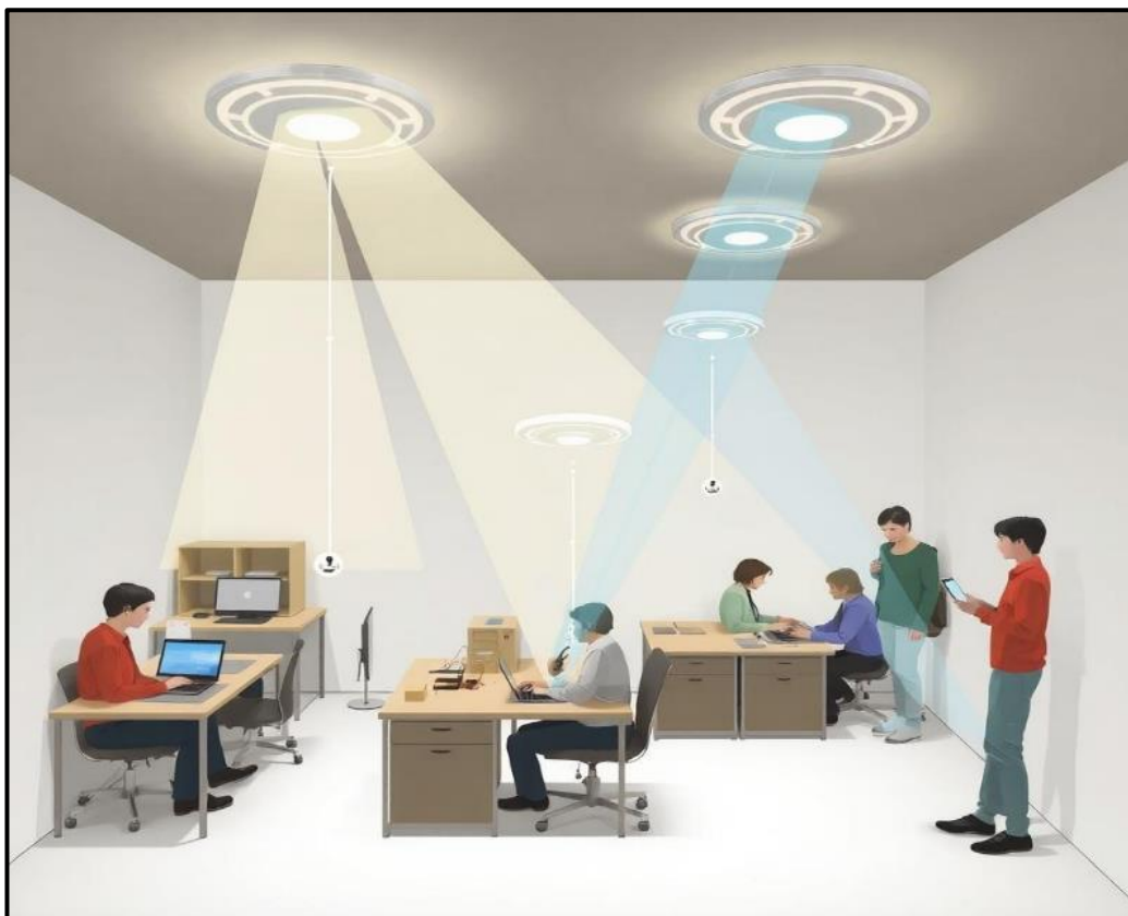
Fig 1: Overview of Indoor Li-Fi Communication System
